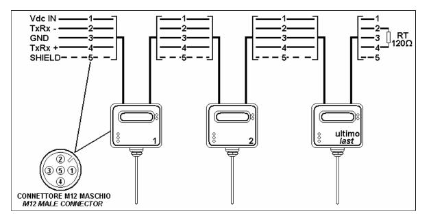
Fit a 120 ohm  $\frac{1}{4}$  Watt terminal resistance to the last device in the chain to reduce serial signal reflections to a minimum: an M12 connector equipped with this resistance (see 'Evoser options') is available for this purpose. Make sure that the master unit (control unit which handles the RS485 network) is equipped with this resistance between the RS485 RxTx+ and RxTx- signals: if it is not so equipped, install one.
