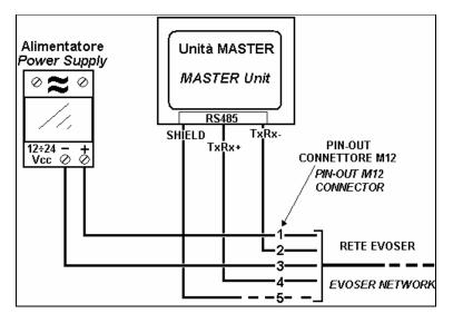
Power the Evoser network with a stabilised power supply with output voltage in the range 12 to 30V DC: voltage in excess of this maximum will cause the entire chain of devices connected to the power supply to fail.
