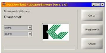
Click on '*Find*' to open the new firmware file (\*.mot) to be written to the Evo Ser device; select the serial port to which the device is connected, and click on '*Program*'.
