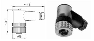
This connector (5 female poles) can be used to cable the Evo Ser network: for further information, see '*Electrical connections*'.
