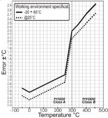
*Note: in the range -50°C to 300°C the accuracy of the Pt1000 sensor is class A; above 300°C the accuracy of the sensor is class B*
