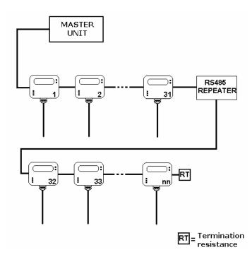
The termination resistances (RT = 120 ohm) are installed at the beginning and end of each segment of network.
